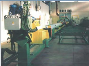
*Cutting machine for polygonal columns*
