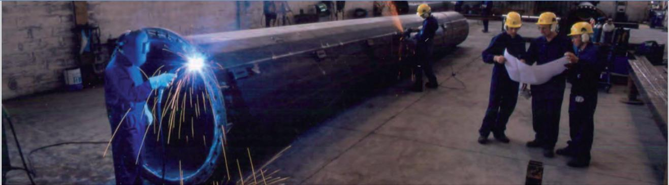
*Automatic welding machine for polygonal columns*
