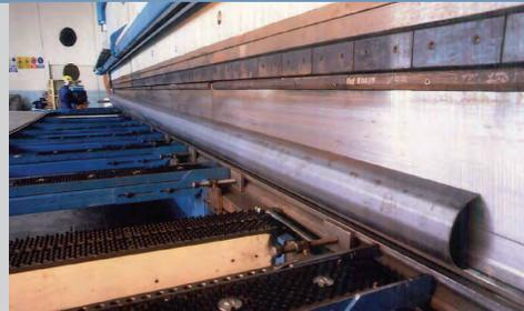
*Second line for conical columns welding*
